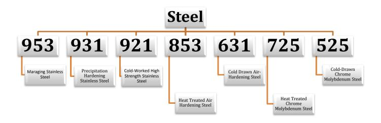
Reynolds branding started with the legendary "531" used for cycle, motorcycle, automotive and aviation use commencing in 1935. For our steel products, the increasing brand number generally indicates higher strength based on the alloy content.
